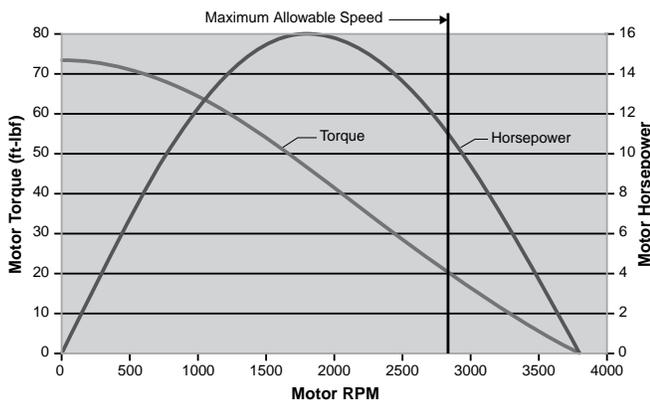
Figure 2: MMP150 Air Motor Performance
